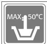
**Symbol of maximum temperature for filling the solution tank:**
