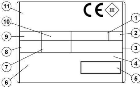
1. The weight of the batteries used to power the appliance (expressed in Kg).
