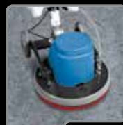
Dry maintenance: stripping and polishing of vinyl floors
